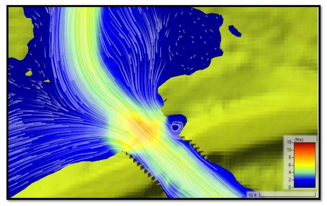
Figure 5. Screenshot from 2D RAS Model with Particle Tracers and Velocity Map for 50% AEP Flow
